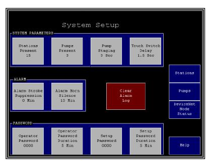
The current passwords are displayed under **Operator Password** and **Setup Password**. A value of **0000** means that no password is required.
